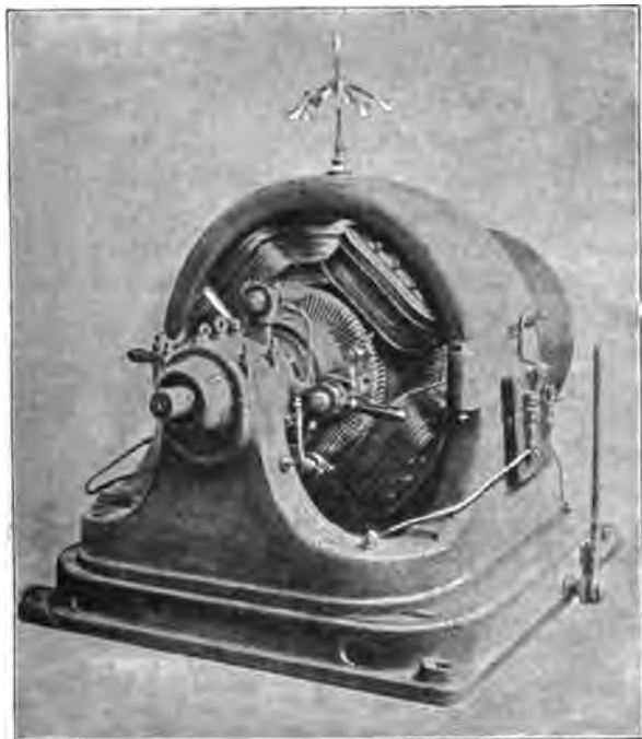
FIG. 10.—CONTINUOUS-CURRENT SELF-EXCITED COMPOUND-WOUND QUADRIPOLE GENERATOR.
